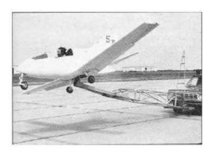
Clockwise from above; the Truck-A-Plane in action, the only known way to receive "flight instruction" on a BD-5; the original two-place BD-10 turbojet; N52BD, Keith Hinshaw's personal BD-5.
