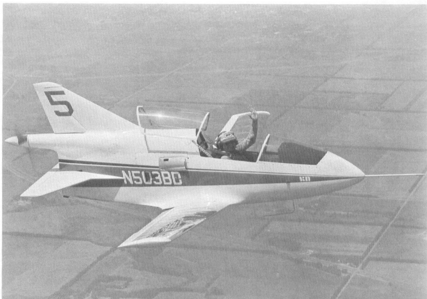
A friendly wave from Berven, BD's Chief Test Pilot at 90 mph shows the ease with which it handles with the canopy open. At 90 mph the BD-5 feels only a slight draft from behind and his baseball cap stays in place.
